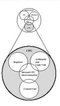
Figure 1.5 The Central Processing Unit (CPU)
