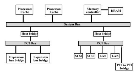
Note: In a multiprocessor system, one or more PCI configurations may be connected by bridges to the processor's system bus.
