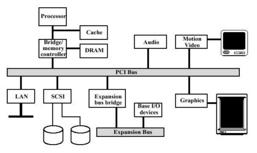
Note: Bridge acts as a data buffer so that the speed of the PCI bus may differ from that of the processor's I/O capability.
