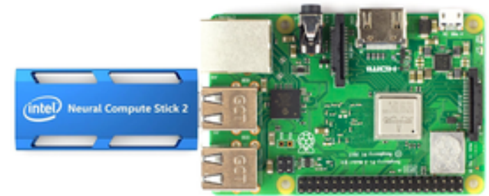
Raspberry Pi 3B + Intel Neural Compute Stick 2
