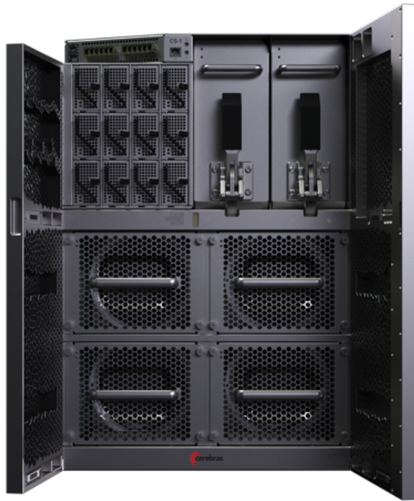
Figure 3: Front view of the CS-1, with doors open. Fans in the bottom half move air; pumps in the top right move water, power supplies and I/O in the top left provide power and data.
