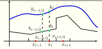
cells  $c_i = [x_{i-1/2}, x_{i+1/2}]$  with centroid  $x_i$  and interface  $x_{i+1/2}$  $h_i^n$ ,  $u_i^n$ ,  $\eta_i^n$ ,  $b_i$  approximations on cell  $c_i$  at time  $t^n$  $W_i^n = (h_i^n, h_i^n u_i^n)$  conservative variables vector
