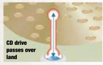
When the laser from a CD drive strikes a land on a disc, most of the light is reflected back to the drive's sensor. The drive knows the laser has passed over a land, due to the high percentage of light reflected back.
