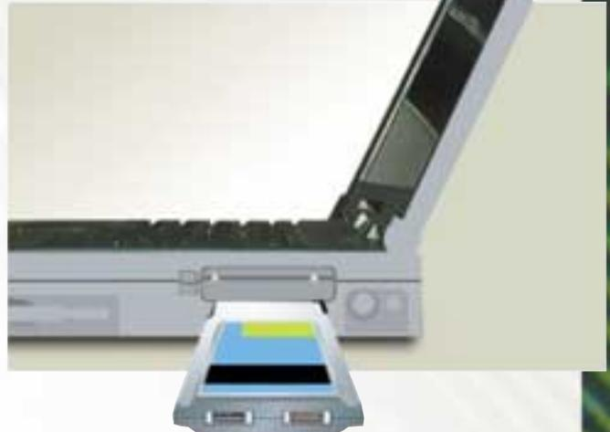
**PC Card Slots:** Installing a PC Card in the PC Card slot of a portable computer is probably the most simple hardware installation you are likely to encounter in personal computing. Simply slide the card into the appropriate slot and the computer's software should detect and configure the card for immediate use.
