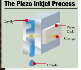
Piezo-electric inkjet printheads work by sending a current through a Piezo crystal. The crystal expands, squeezing ink out and onto the paper.
