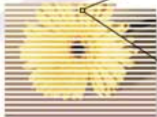
A graphics program saves the image line by line, from the bottom to the top.
