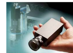
Smart Camera System (120x50x35 mm) (250g)
