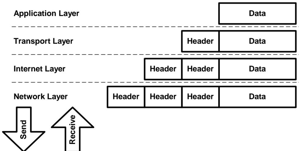
**Figure 2. Data Encapsulation**
