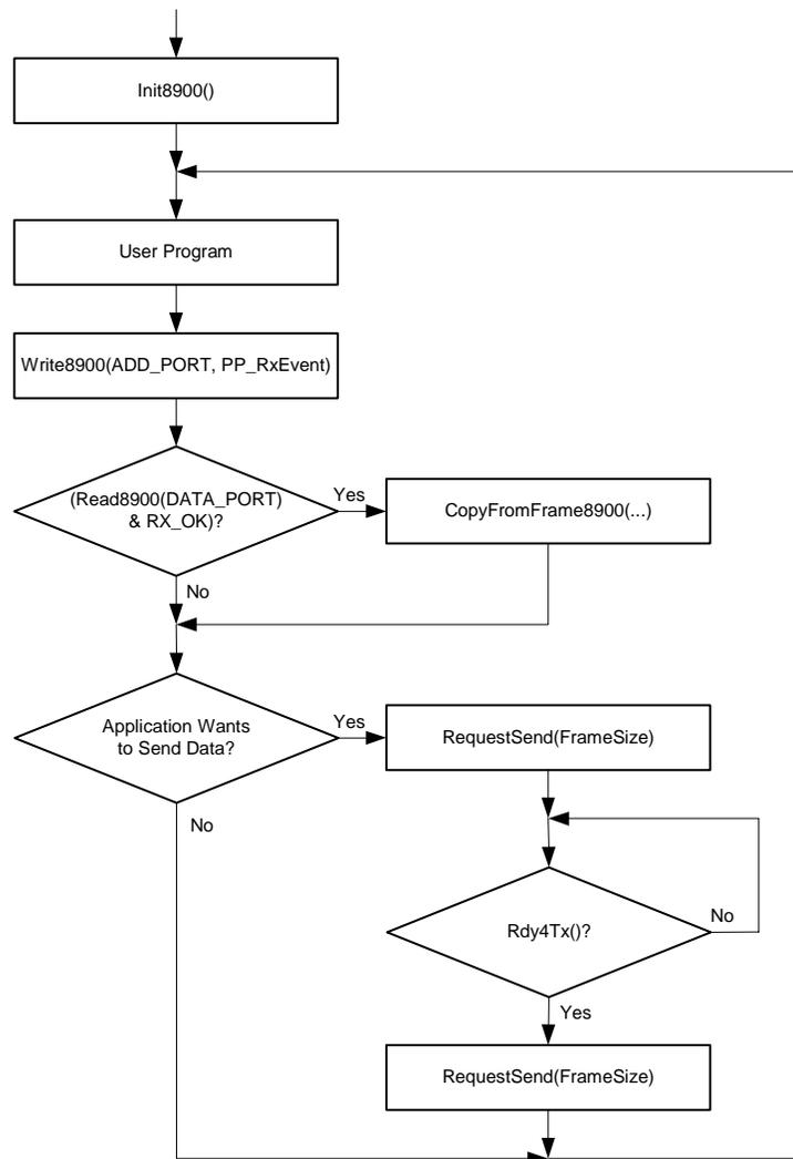
Figure 5. Using the Ethernet Module
