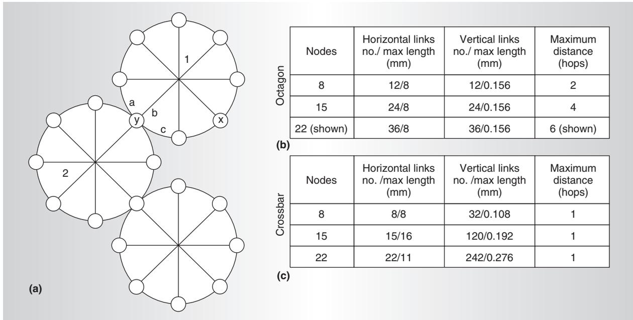
Figure 7. Scaling strategy 1. Bridge nodes (node *y*) connect adjacent Octagons (a) and perform hierarchical packet routing. Member nodes attach to only one Octagon (node *x*). The tables give the maximum distance for Octagon (b) and crossbar (c) networks of various sizes.
