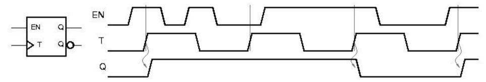
D and J-K flip-flops can be used to build a T flip-flop with enable.
