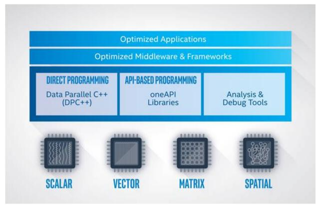
As shown in the figure above, applications that take advantage of the oneAPI programming model can execute on multiple target hardware platforms ranging from CPU to FPGA. The oneAPI product is comprised of the Intel® oneAPI Base Toolkit and several add-on toolkits featuring complementary tools based on specific developer workload needs. The Intel oneAPI Base Toolkit includes the Intel® oneAPI DPC++ Compatibility Tool, select libraries, and analysis tools.
