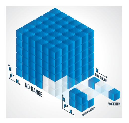
When kernels are executed, the location of a particular work-item in the larger ND-range, work-group, or sub-group is important. For example, if the work-item is assigned to compute on specific pieces of data, a method of specification is necessary. Unique identification of the work-item is provided via intrinsic functions such as those in the nd item class (global id, work group id, and local id).
