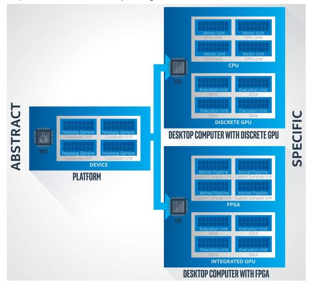
The platform model is general enough to be mapped to several different types of devices and lends to the functional portability of the programming model. The hierarchy on the device is also general and can be mapped to several different types of accelerators from FPGAs to GPUs and ASICs as long as these devices support the minimal requirements of the oneAPI programming model. Consult the oneAPI Release Notes for more information.
