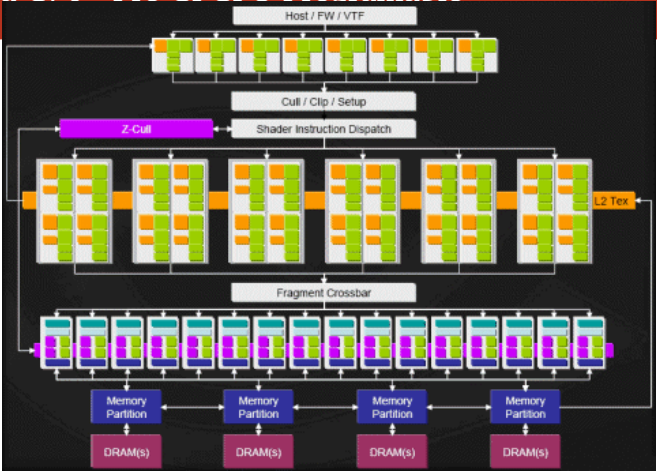
Figure: NVidia G70 Architectural diagram (source NVidia)
