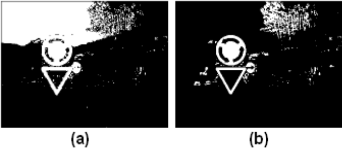
Figure 8: Segmentation (a) Hue/Saturation (b) Hue/Chromatic
