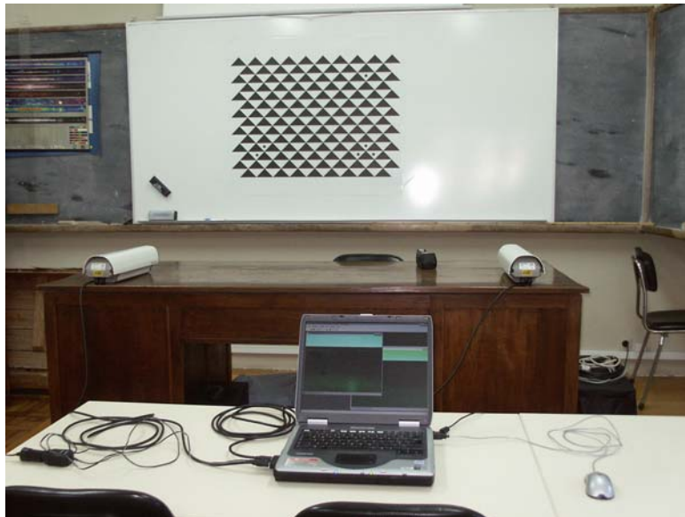
Figure 3: Image acquisition to obtain calibration parameters of the video camera lenses.
