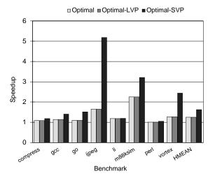
Figure 2. Optimal STP Speculation on Single-Level Loops
