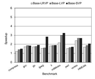
Figure 9. Speculating both Loops and Procedures on a 4-way STP Machine with Rollback
