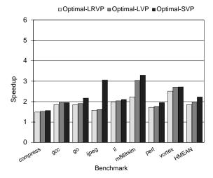
Figure 7. Speculating both Loops and Procedures on a 4-way Optimal STP Machine
