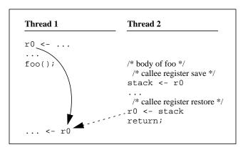
Figure 1. Dependences Induced by Callee-Saved Register Operations
